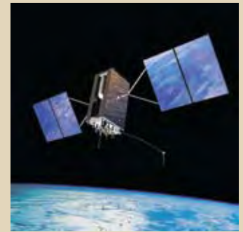
Figure 5 GPS III will improve position, navigation and timing services for military troops and civilian users worldwide with anti-jam capabilities.
